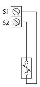
Configured for remote room sensor or limit sensor
